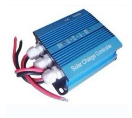
Battery State-of-Charge display with 3 LEDs; Acoustic load disconnect pre-warning; PWM-regulation (series type); Boost, Equalize and Float charging, also for VRLA; Automatic 12/24 Volt detection; Integrated temperature compensation; Large terminals (up to 6mm2 wire size); SOC and voltage controlled LVD; Fully electronically protected.
